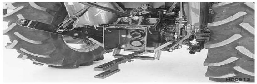
The drawbar can move from side to side and fore and aft. See Field Operation section in this manual for Drawbar Preparation.
