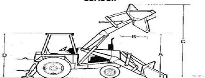
NOTE: Specifications taken with 74" (1880 mm) short lip loader bucket, 14.9 x 24 - 6PH rear tires and 7.50 x 16 - 10 PR front tires.
