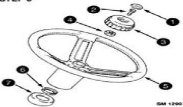
Remove the emblem (1), bolt (2) cover (3) and retaining nut (4). Using a suitable steering wheel puller and remove the steering wheel (5), retaining ring (6) and collar (7).
