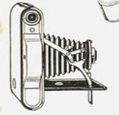
Be sure the Struts are fully extended and locked in position. The camera is closed by pressing downwards with your two thumbs on the centres of the Struts.
