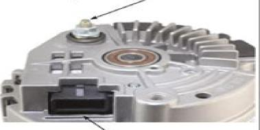
When using with OEM wiring harness, plug in factory connector here
