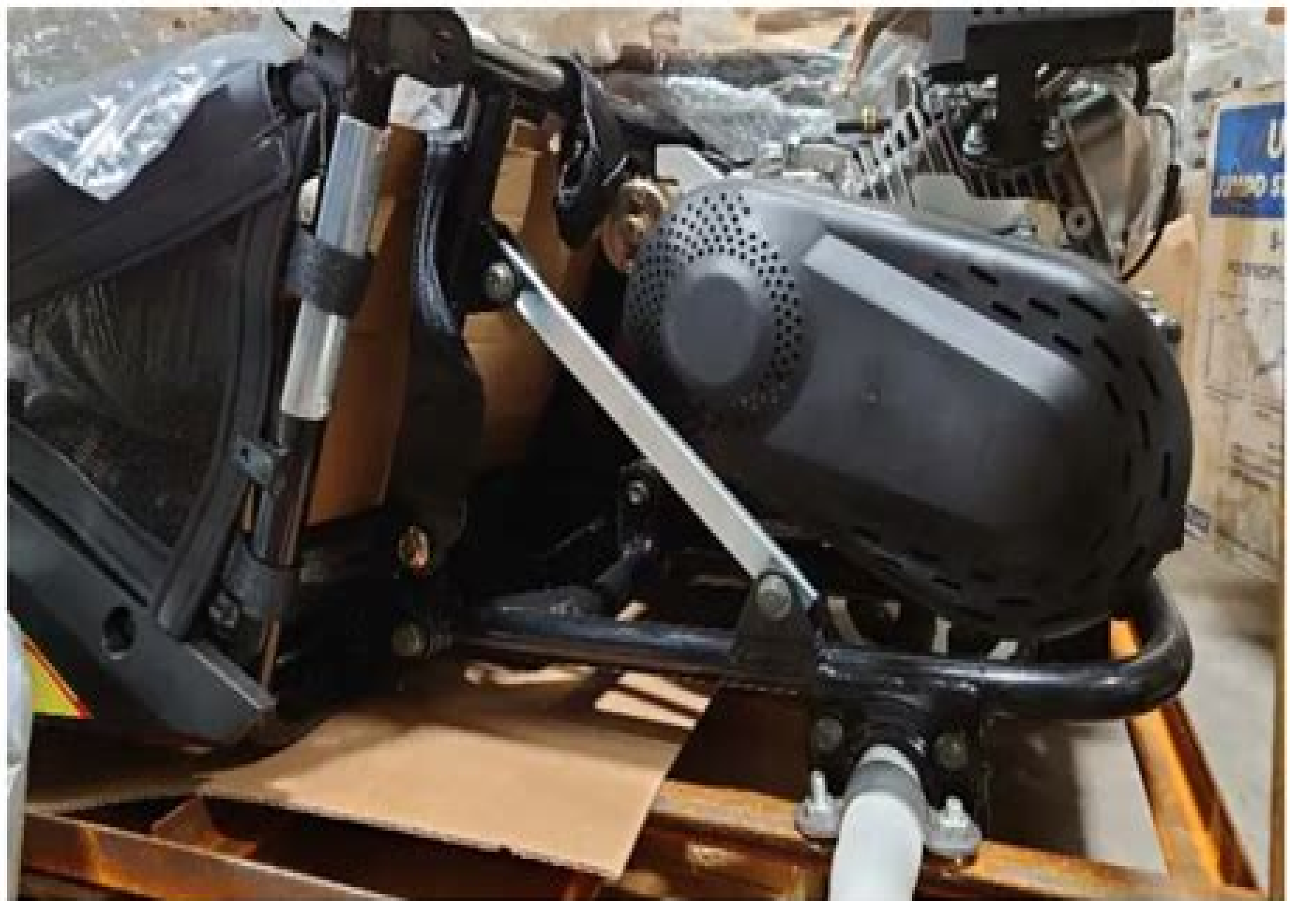
Figure 1.4: Remove Rear Support Arms
