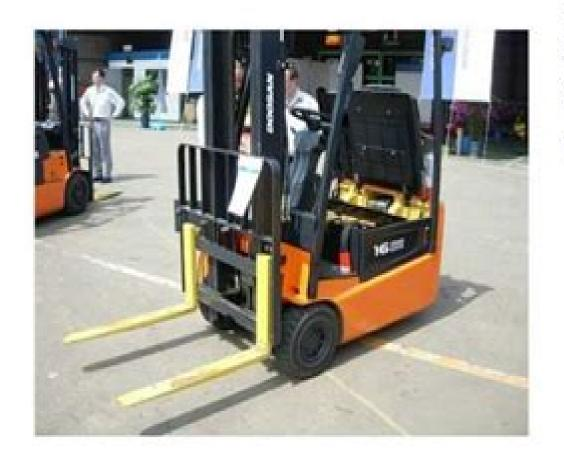
24 VOLT REAR WHEEL DRIVE SOLID SOFT TIRE 2400 TO 3000 LB CAPACITY OCDB STANDARD NEW ORANGE COLOR
