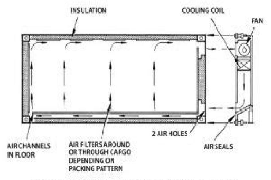
Insulated container requiring external refrigeration source. Bottom air delivery.
