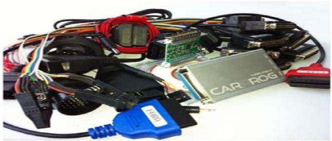
CARPROG was designed with regard to demands of our customers to have universal tool for car radios, odometers, dashboards, immobilizers repair including advanced functions like EEPROM and microcontroller programmer, key transponder programmer.
