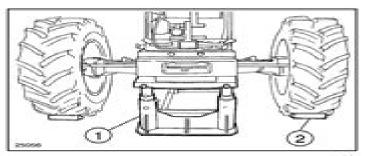
Insert tool 295022 (1) in the clutch center hole.
