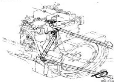
If equipped with a heater, open the heater coolant valves on the engine.
