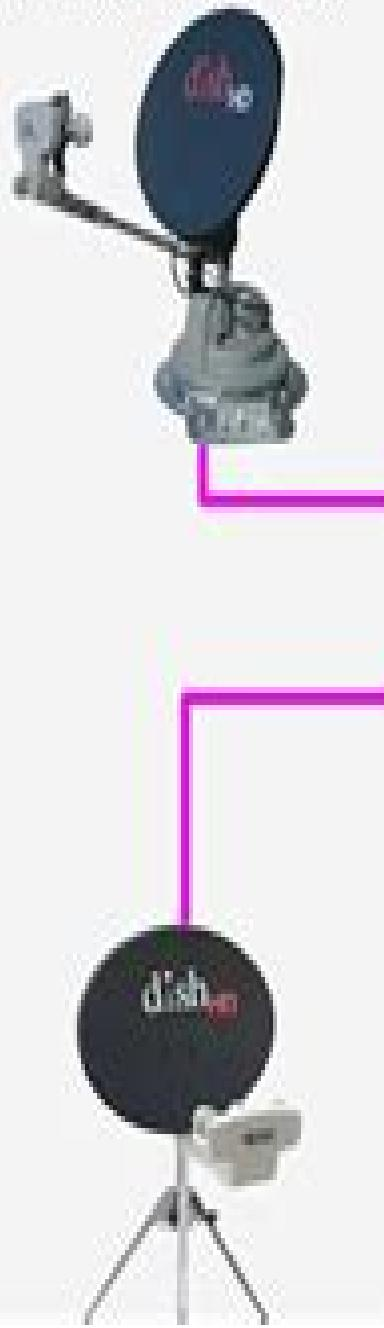
During the time when the Winegard Travler is acquiring satellites, the Hopper 3 can not be connected to the Travler. Otherwise, there is a good chance that a fatal "No LNB Voltage" error will occur.
