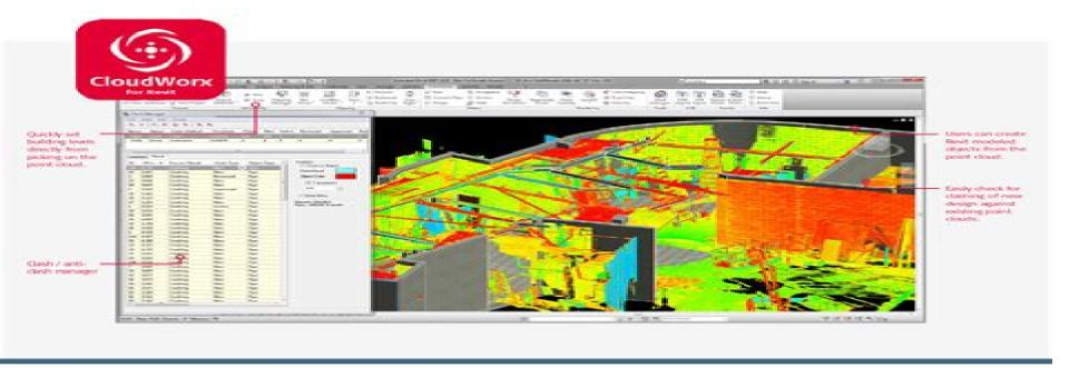
Lesca CloudWork for Revit is a breakthrough plug-in for efficiently using rich as-built point cloud data, captured by laser scanners, directly within Revit for simpler and faster BIM modeling of existing buildings. This is useful for a wide range of BIM activities including retrofit design, construction and operations, and lifecycle asset management of the building. It provides a virtual visit to the site within Revit with a complete view of the captured reality.
