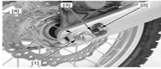
Push the wheel forward and derail the drive chain [1] from the driven sprocket.
