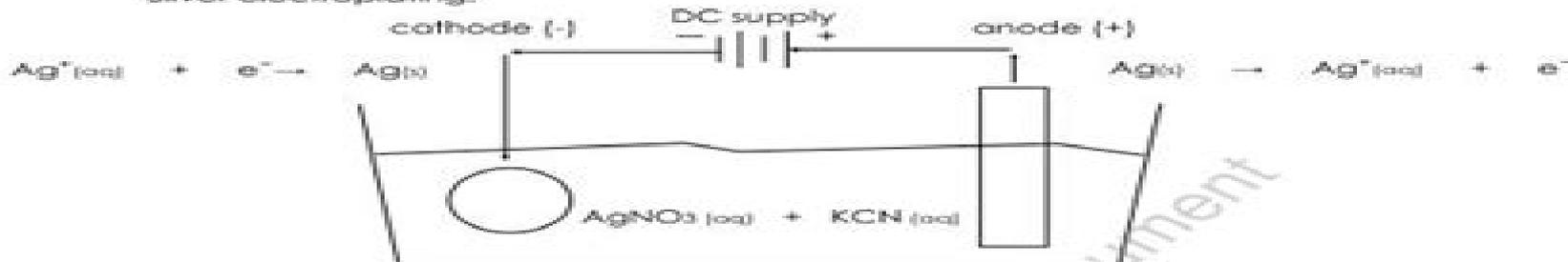
The mass of the silver electrode at the anode decreases over time as a thin silver layer forms on the object at the cathode
