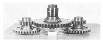
Place both countershafts against the autput shaft, meshing the marked booth on each countershaft between two of the marked teach on the low speed gear.
