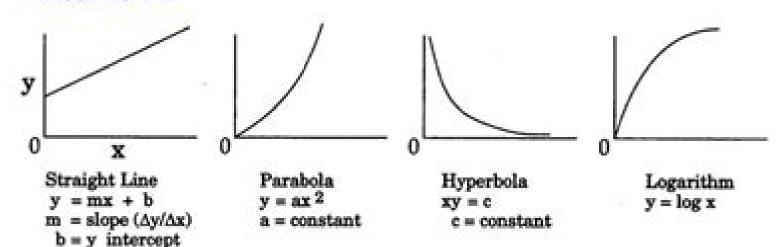
Figure 39. Common curves encountered in laboratory experiments.
