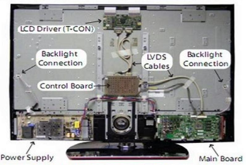
T-CON - CONTROL BOARD - POWER SUPPLY - MAIN BOARD
