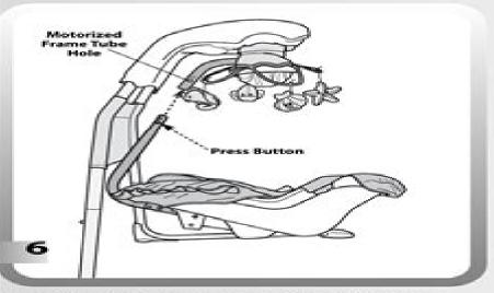
Press the button on the seat tube and slide the seat tube into the motorized frame tube. Make sure the button on the seat tube "snaps" into the larger hole in the motorized frame tube.
