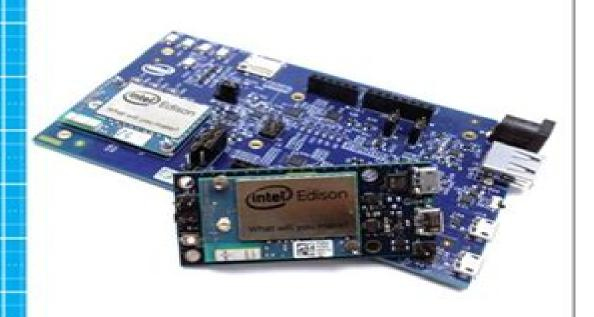
Sensors, Actuators, Bluetooth, and Wi-Fi on the Tiny Atom-Powered Linux Module Stephanie Moyerman
