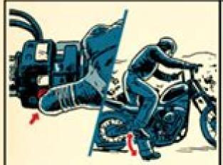
Start the bike by switching the key to the "On" position and either pressing the ignition button or using the kickstart lever.
