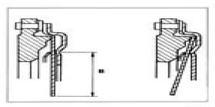
Partial section of "thrust" clutch (for 1370 - 1580 - 1747 - 1998 20v - 1910 TD segines)
